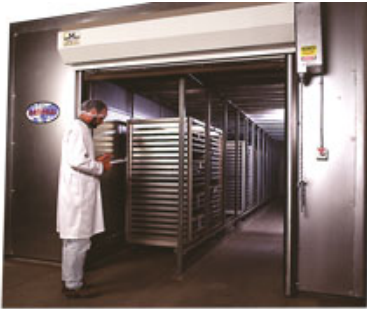
BioWorld Microbes are grown and dried for easy storage, long shelf life and safe handling.
