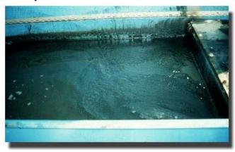
3 days after BioWorld Hydrocarbon Treatment, the thick oil was degraded to a fine layer of fatty acids. (The unit was moved outside.)
