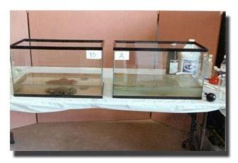
Oil Sludge from old well drilling pit. Side by side comparison. (See dried lump in tanks.)
