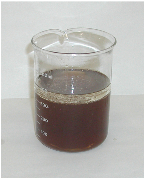
Figure 3—Blanket 510 floats on top of liquid.
